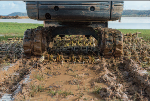
Ground Rolls provide fantastic surface protection - illustrated here with and without the ground roll
